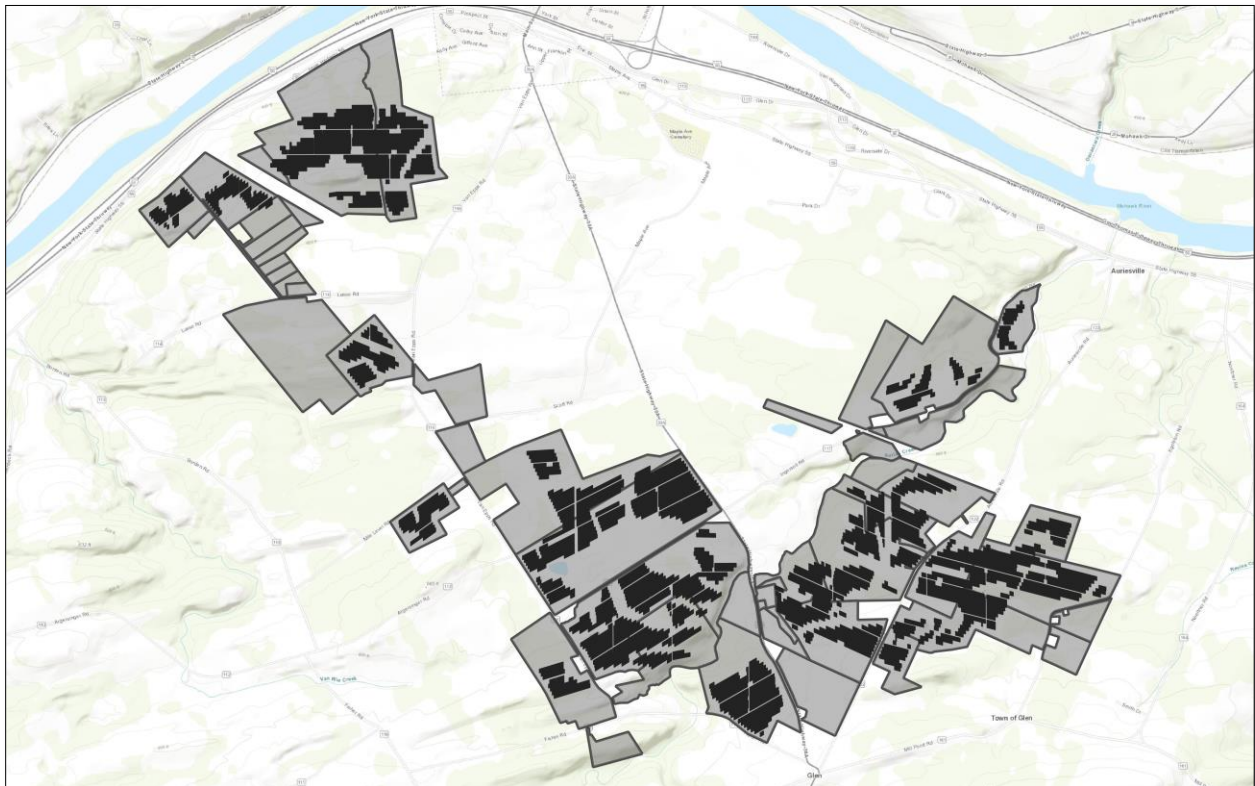
Figure 1: Mill Point Solar I Project land parcel boundaries (gray) with PV panel layout (black)
